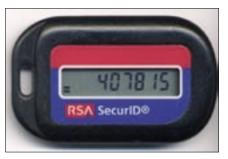
Figure 1: The RSA Security keyfob displays a new six-digit number every 60 seconds.
