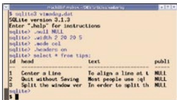
Figure 3: The tips are stored in an SQLite database. With just a couple of formatting instructions, the client will display the table in a readable way.
