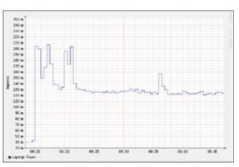
Figure 4: Power consumption of a laptop shortly before and after switching on.
