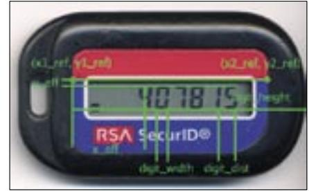
**Figure 5: The two reference points (x1\_ref, y1\_ref) and (x2\_ref, y2\_ref) at the top corners of the blue area determine the coordinate system from which the pixel distances for the individual digits are generated.**
