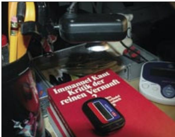
Figure 2: My Fobcam lab setup: a lamp ensures constant light, and the webcam is perpendicular to the SecurID token.
