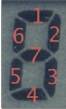
**Figure 4: Numbering the segments in the LCD display helps define the logic for the simple character recognition algorithm.**
