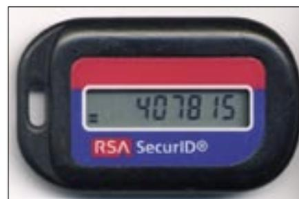
Figure 1: The RSA Security keyfob displays a new six-digit number every 60 seconds.
