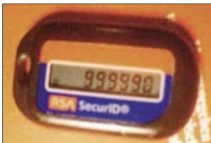
Figure 3: The OCR system has correctly identified the number in the display. The OCR mask is attached to the two green reference points; sensors are placed at the positions marked in red to scan the numeric output.
