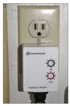
Figure 3: The X10 receiver, with the aquarium pump's power cable plugged in.
